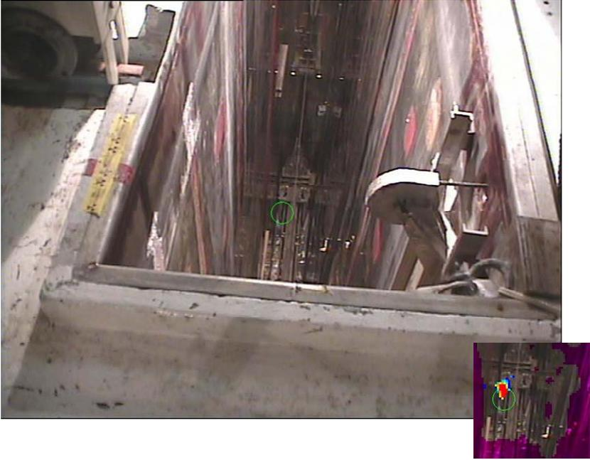
**Figure 4. Full Size View of the Location of the Most Elevated Dose and Count Rate Found In Survey 1**
