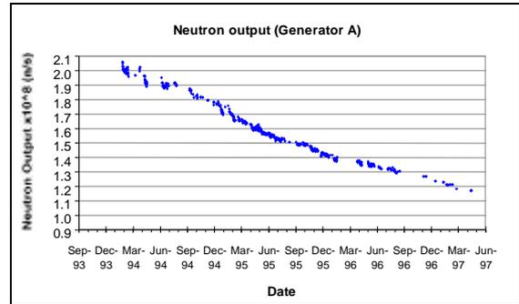
**Figure 5** Reduction of Sodern Genie-26 deuterium-tritium neutron generator output with time.
