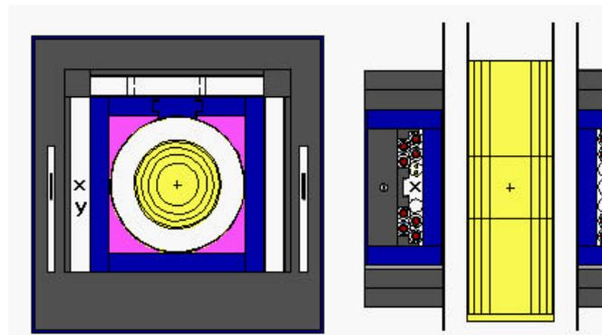
**Figure 7** MCNP model of the Hulls Monitor.
