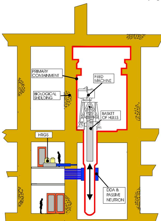
**Figure 1** Schematic Arrangement of the Hulls Monitor.
