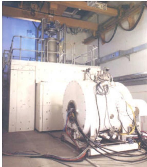
**Figure 8** Radiometric Development Facility pulsed superconducting cyclotron and Advanced Fuels Hulls Monitor development rig.
