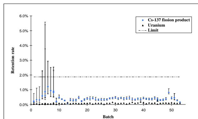
**Figure 4** Residual Fuel and  $^{137}\text{Cs}$  Retention in BWR Hulls Batches.
