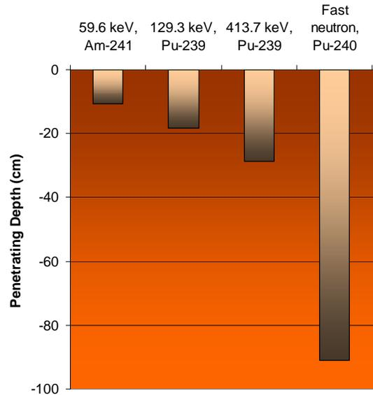
Figure 1. Radiation penetration depths in soil
