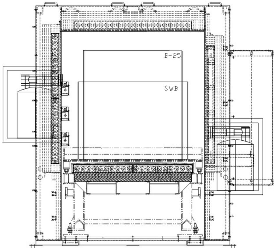
Figure 3 Cross sectional view of the mid-section of the assay cavity showing the neutron detectors, neutron generator and gamma detectors
