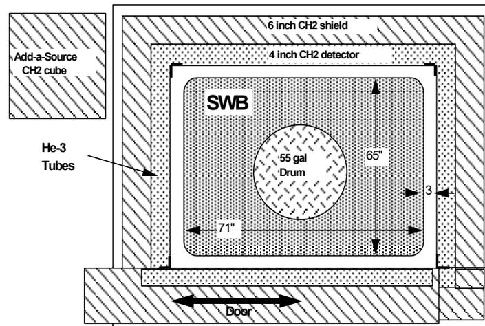
**Fig. 2. Diagram of the SuperHENC detector body**
