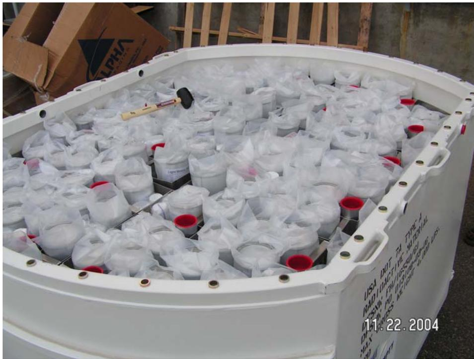
**Figure 2.** Test SWB used during the SuperHENC calibration confirmation showing the interfering matrix material and a grid of insert tubes for loading of the Pu sources.
