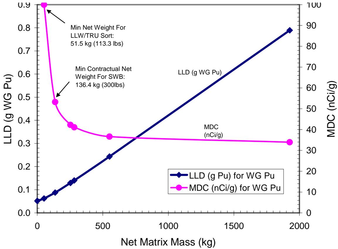
**Figure 3.** Neutron LLD and MDC plot against net matrix mass.
