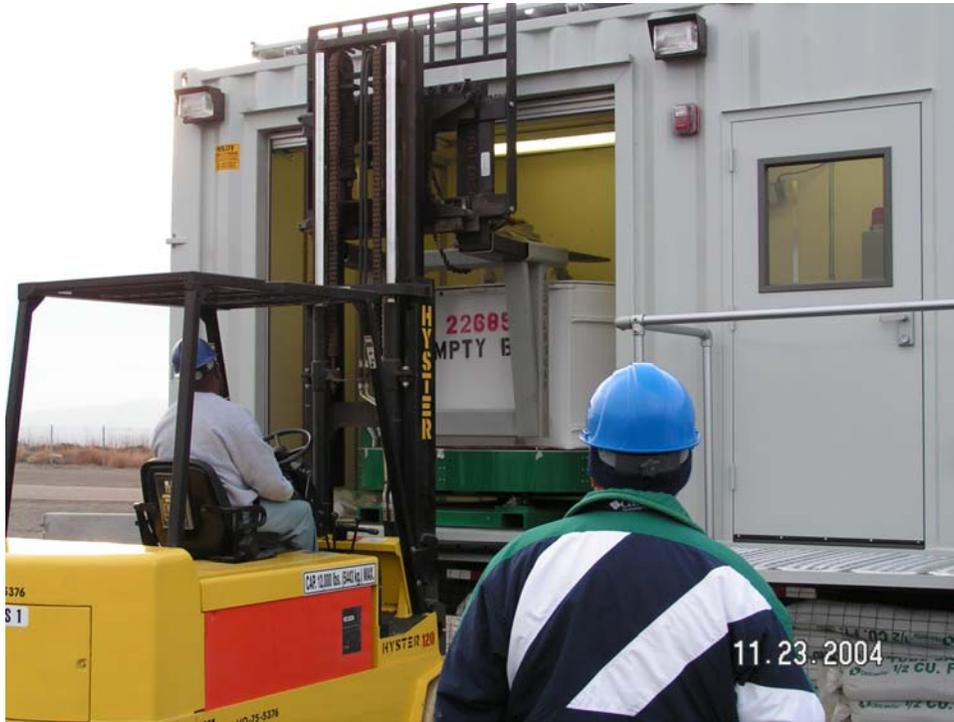
**Figure 1.** Test SWB being loaded on the gamma turntable using a fork lift fitted with special attachment designed for handling SWBs.
